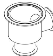
Lower Body L, 2 ports L型雙口体 SS316
